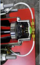
The inflation system can keep the tires properly inflated by using compressed air from the trailer's air system to inflate any tire that falls below a preset pressure whenever the vehicle is in operation.
